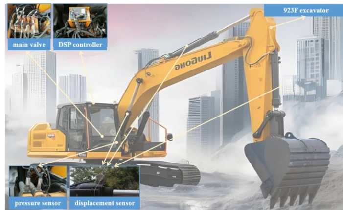
Figure 6. Robotic excavator trajectory control experimental platform.
