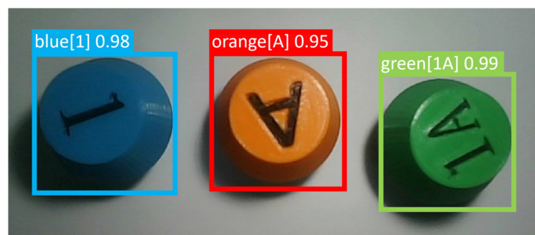
Figure 5. Material category recognition based on the YOLO algorithm.
