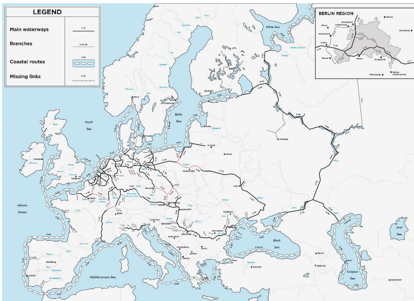
Figure 1. Map of the potential pan-European inland waterway network showing how the E40 waterway between the Baltic and the Black Sea could function—the only problem is the absence of crucial connections between watercourses: the missing links are marked with dotted lines on the map. Furthermore, this system can integrate the water transport networks of Belarus and Ukraine with the EU (Source: redrawn and modified after https://unece.org/ accessed on 8 January 2022).
