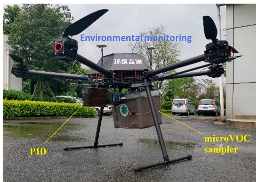
Figure 1. The environmental monitoring UAV with attached PID and microVOC sampler.
