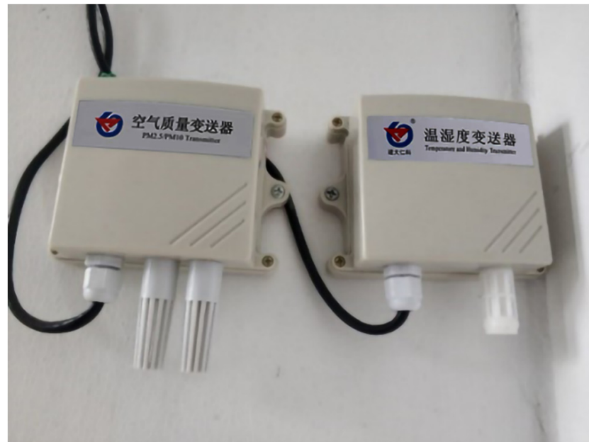
Figure 2. Air quality transmitter and temperature & humidity transmitter.
