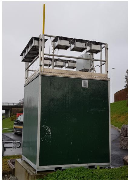
**Figure 1.** The roadside Schancheholen air quality monitoring station (station ID NO0125A), operated by Stavanger municipality, with the ten AirSenseEUR units mounted on top. Photo credit: Rolf Haugen.
