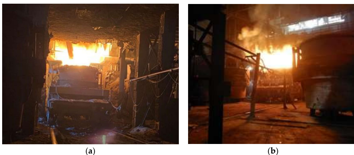
Figure 2. Tapping period of electric furnace. (a) Early stage of tapping. (b) Late stage of tapping.
