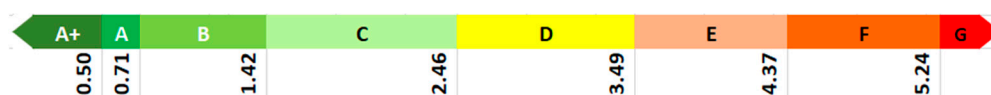
Figure 4. Energy scale for one hour of heating, valid for the studied space, in kWh.
