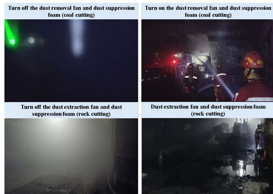
Figure 19. Comparison of visibility at the cutting face before and after turning on the dust extraction fan and foam.
