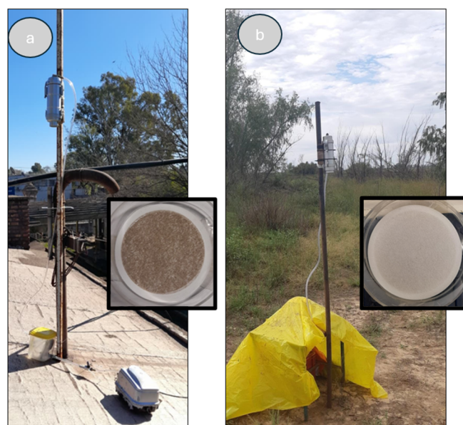
Figure 3. Harvard impactors installed at measurement sites and Teflon filters (embedded figures) after collecting PM_{2.5} during a sampling period at each corresponding site. (a) Site 3 (port-urban), winter campaign, filter sampling period 26–29 July 2021. (b) Site 9 (natural), summer campaign, filter sampling period 2–8 March 2022.
