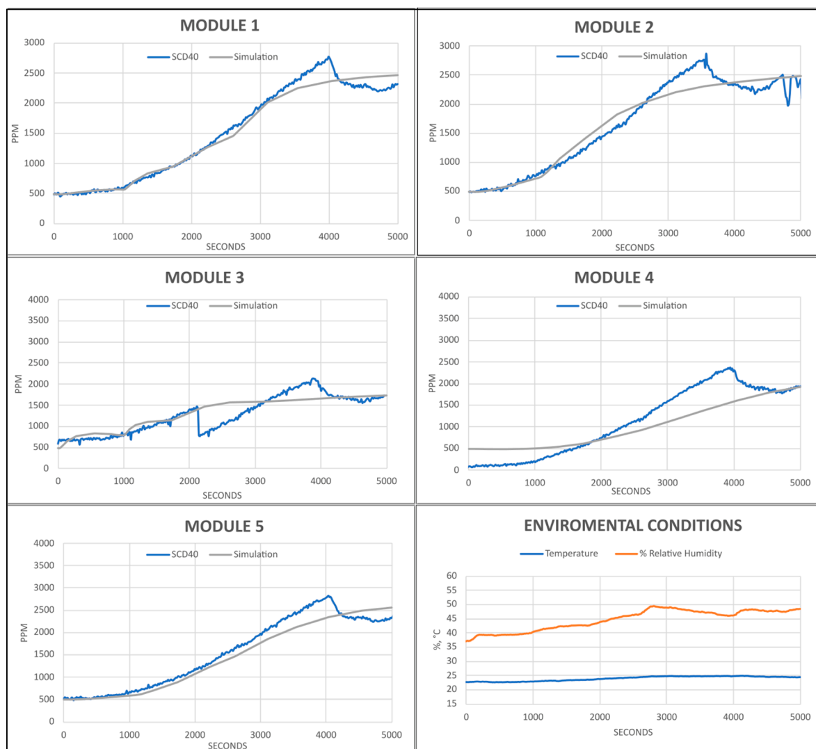
Figure 11. SCD40 data vs. CFD simulation.
