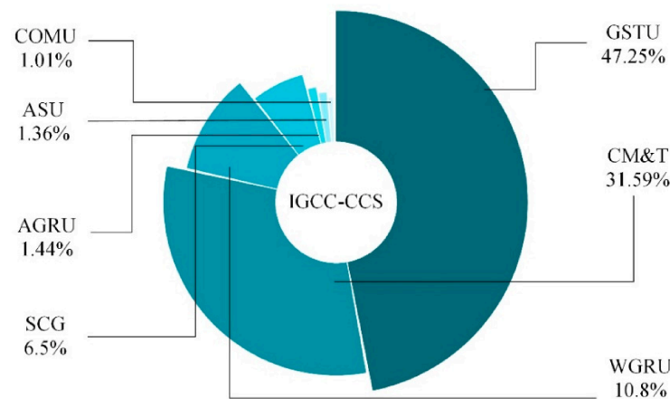
Figure 9. Exergy loss distribution of different sub-units in the IGCC-CCS plant.
