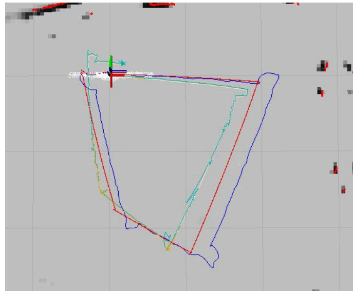
Figure 22. RTAB-Map and IMU odometry fusion with the EKF trajectory in Rviz.
