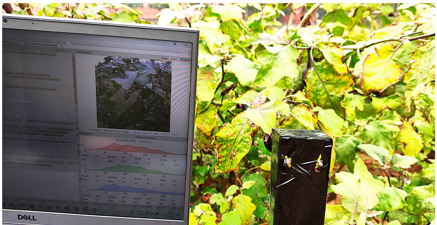
Figure 12. Real-time field deployment of the proposed FOMO detector on OpenMV Cam H7.
