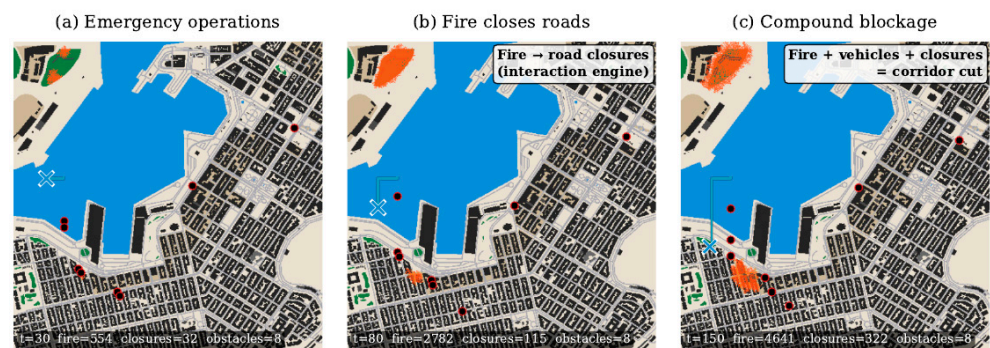
Figure 5. Fire–obstacle coupling on the Piraeus topology (illustrative seed s = 42 ; benchmark seeds are \{0, \dots, 29\} ). (a) t = 30 . (b) t = 80 . (c) t = 150 . The basemap shows the port topology in its natural colours (blue water, grey built-up area, green vegetation); orange denotes the burning cells, dark red discs the emergency vehicles, the teal line the executed route and the blue cross (x) the UAV. The overlay in each panel reports the step index together with the fire-cell, road-closure and obstacle counts.
