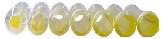
Figure 3. Constructed phantoms used for designing various void fractions.
