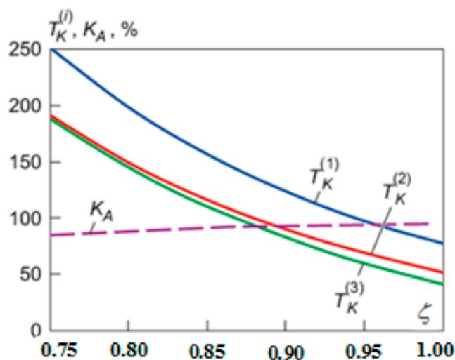
**Figure 14.** Dependence of the readiness coefficient and the TIBV on the total production capacity of metrological units.
