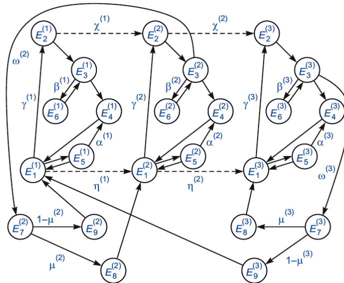
Figure 10. Graph of the model of operation, degradation and renewal of the CTS fleet with incomplete resource recovery.
