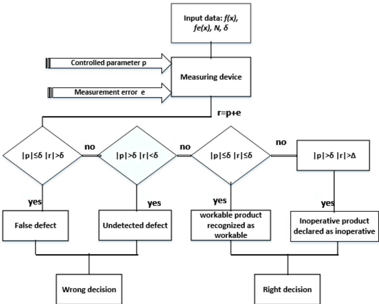
Figure 3. General scheme of diagnostics and decision-making based on the tolerance control method.
