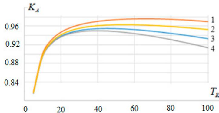
**Figure 2.** Dependences of the readiness coefficients on the periodicity of the control for various distribution laws: Rayleigh’s law (1), normal law (2), exponential law (3), and Weibull’s law (4).
