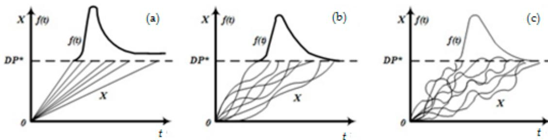
Figure 6. The model of a random degradation process and a scheme for the formation of a time-to-failure distribution: (a)  $\alpha$  distribution (fan process); (b) DN distribution law; (c) DM distribution law.
