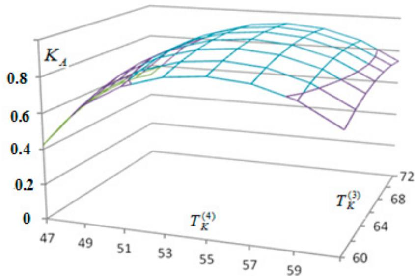
Figure 9. Dependence of the readiness coefficient  $K_A$  on the TIBV for technical conditions  $E_3$  and  $E_4$ .
