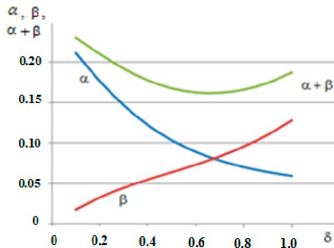
**Figure 4.** Dependences of the probability of an erroneous decision ( $\alpha + \beta$ ), as well as the probabilities of false and undetected failures on the value of the reduced tolerance  $\delta$  on  $z = 0.5$ .
