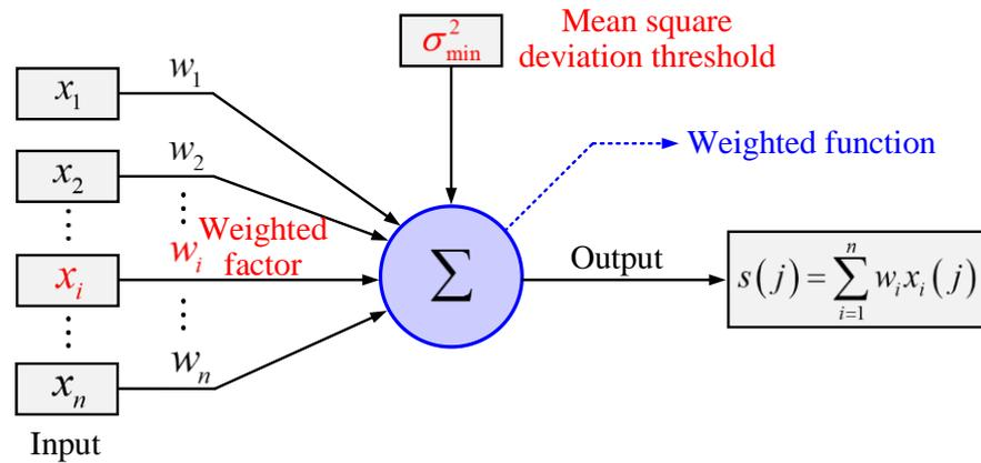
Figure 6. Minimum mean square variance weighted fusion for multi-sensor data.
