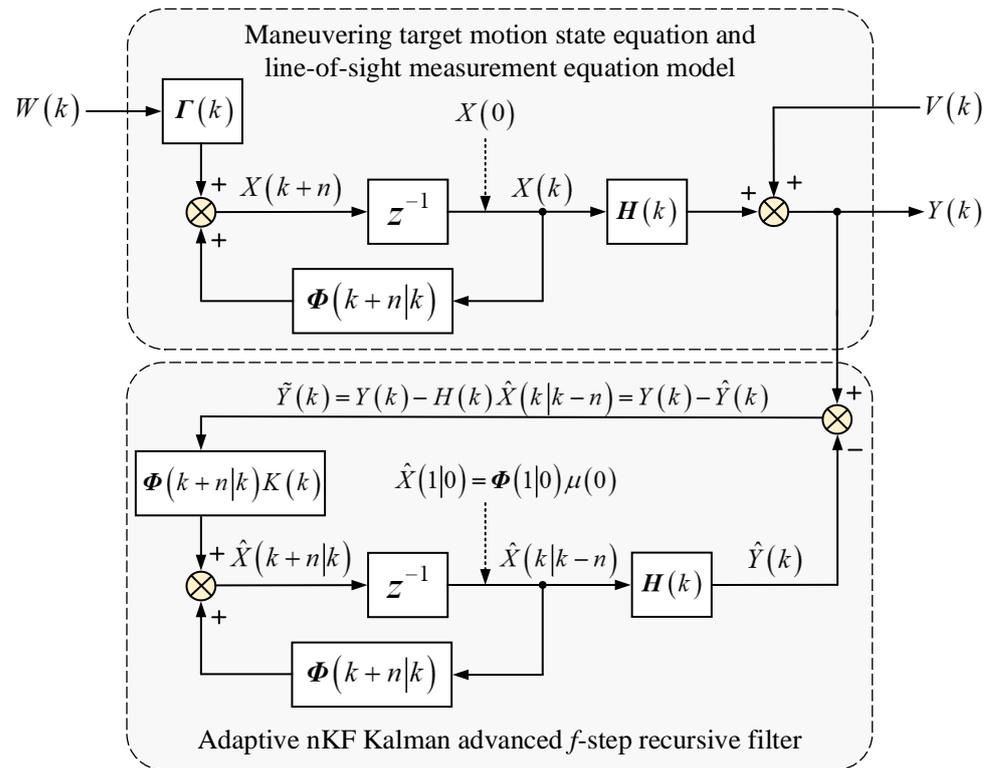
Figure 5. Adaptive nKF Kalman filtering prediction model.
