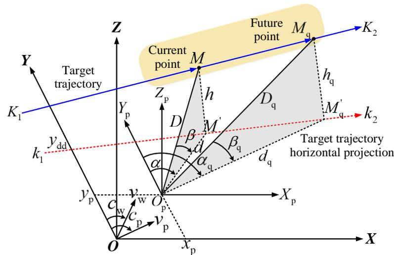
**Figure 2.** Targeting error coordinate system for a “low, slow and tiny” moving target.
