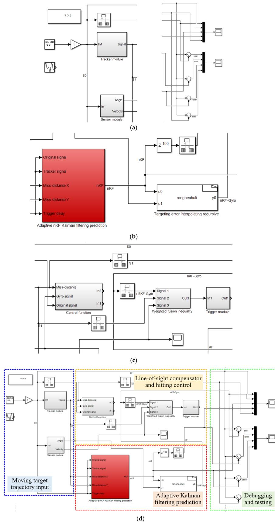
**Figure 8.** Simulink algorithm for targeting control. (a) Moving target trajectory input and debugging testing. (b) Adaptive Kalman filtering prediction. (c) Line-of-sight compensator and targeting control. (d) Overall mathematical control model.
