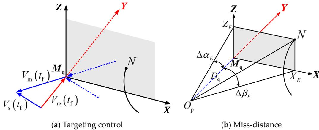
Figure 1. Bullet–target error coordinate system.
