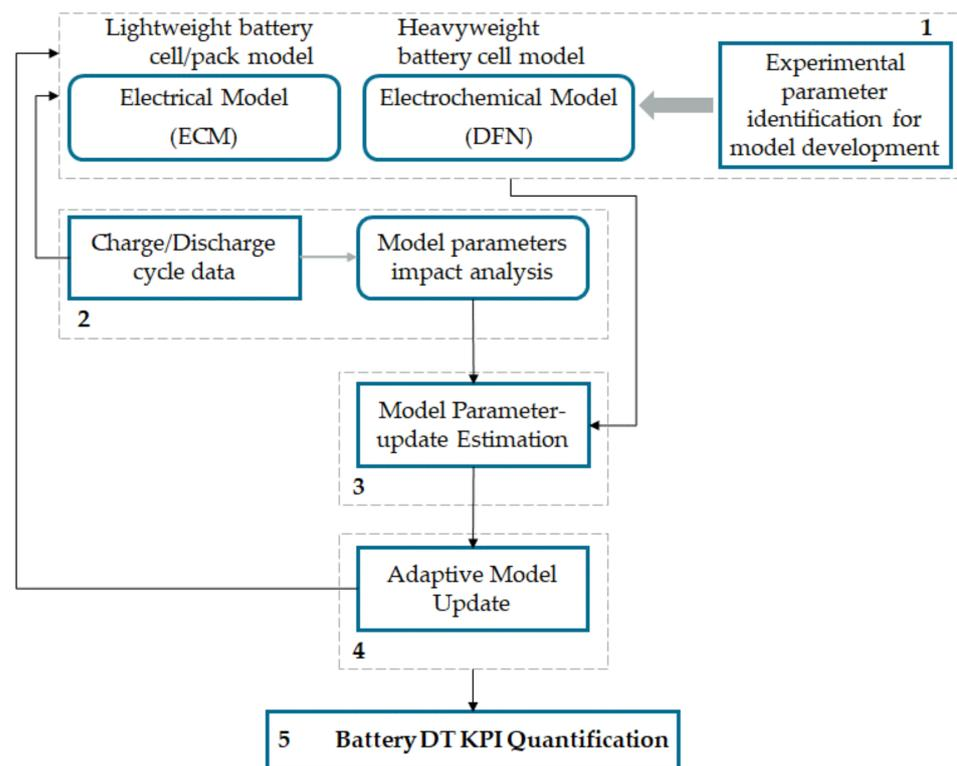
**Figure 2.** Approach for battery DT implementation.
