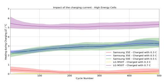
**Figure 8.** Development of the maximum temperature rise during the charging process of the cycle test of the high-energy cells. Solid lines represent the mean values, shaded areas represent the spread of the measured values.
