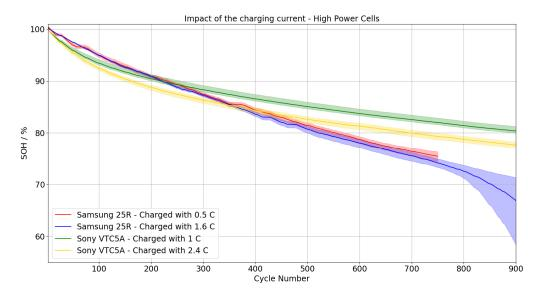
method, while the spread of the cells charged with the standard charge method is less then 1% after 500 cycles.
