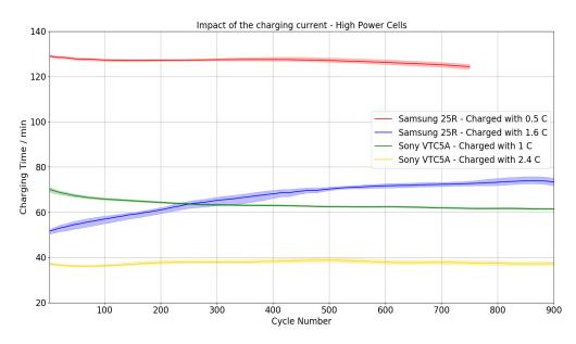
**Figure 5.** Development of the charging times during the cycle test of the high-power cells. Solid lines represent the mean values, shaded areas represent the spread of the measured values.
