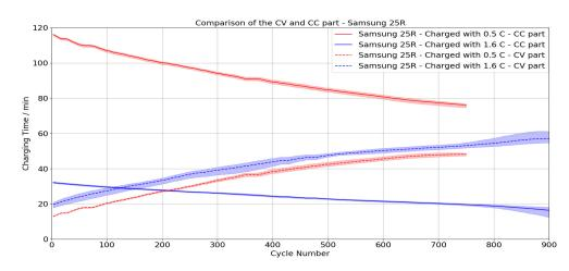
**Figure 13.** Development of the charging time during the cycle test. Separation of the CC and CV part for Samsung 25R.
