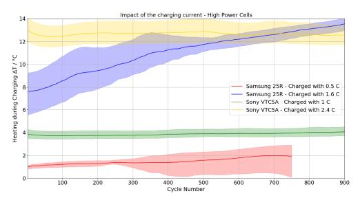
**Figure 7.** Development of the maximum temperature rise during the charging process of the cycle test of the high-power cells. Solid lines represent the mean values, shaded areas represent the spread of the measured values.
