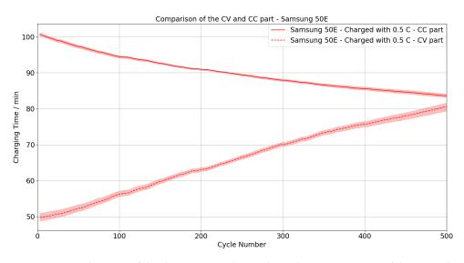
**Figure 12.** Development of the charging time during the cycle test. Separation of the CC and CV part for Samsung 50E.
