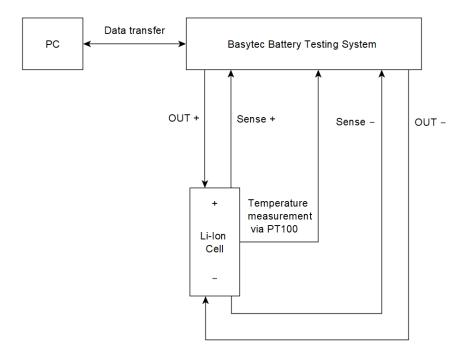
**Figure 1.** Schematic of the measurement circuit for the lithium-ions cells with battery testing system and four wire method.
