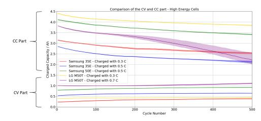
**Figure 10.** Development of the capacity charged during the cycle test. Separation of the CC and CV part for high energy cells.
