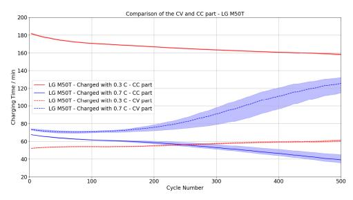
**Figure 11.** Development of the charging time during the cycle test. Separation of the CC and CV part for LG M50T.
