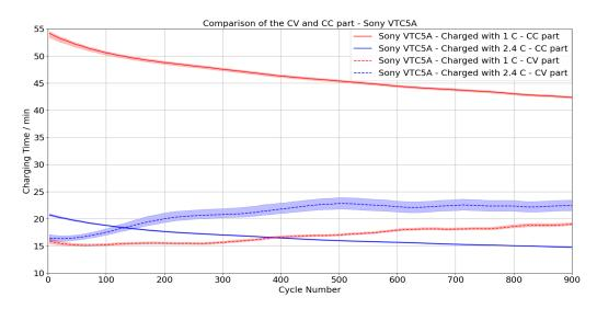
**Figure 15.** Development of the charging time during the cycle test. Separation of the CC and CV part for Sony VTC5A.
