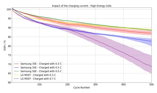
**Figure 4.** Development of the SOH during the cycle test of the high-energy cells. Solid lines represent the mean values, shaded areas represent the spread of the measured values.
