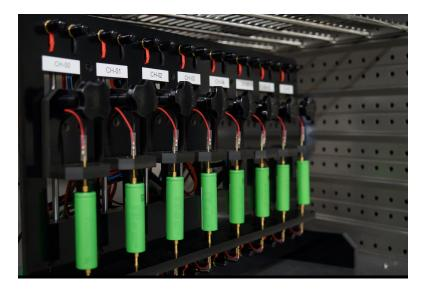
Figure 2. Cylindrical lithium-ion cells connected via cell holder.
