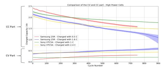
**Figure 9.** Development of the capacity charged during the cycle test. Separation of the CC and CV part for high power cells.
