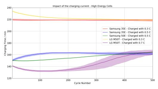
**Figure 6.** Development of the charging times during the cycle test of the high-energy cells. Solid lines represent the mean values, shaded areas represent the spread of the measured values.
