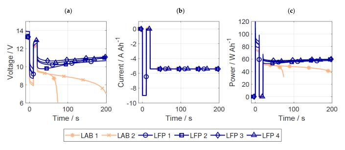
**Figure A2.** Complete cold-cranking test at -10 °C: (**a**) voltage, (**b**) current, and (**c**) power.
