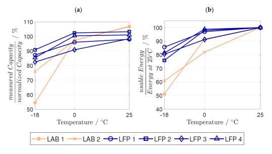
Figure 2. C<sub>20</sub> capacity test (a) measured capacity and (b) useable energy.
