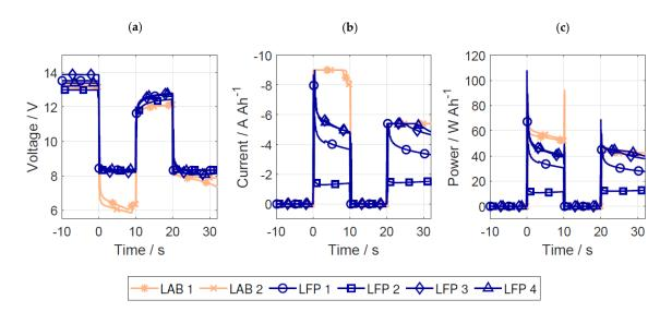
Figure 5. First pulse of the cold-cranking test at -30 °C: (a) voltage, (b) current, and (c) power.
