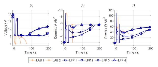
Figure 10. Complete cold-cranking test at -30 °C: (a) voltage, (b) current, and (c) power.
