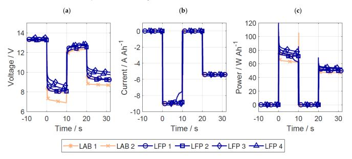
**Figure 4.** First pulse of the cold-cranking test at -18 °C: (**a**) voltage, (**b**) current, and (**c**) power.
