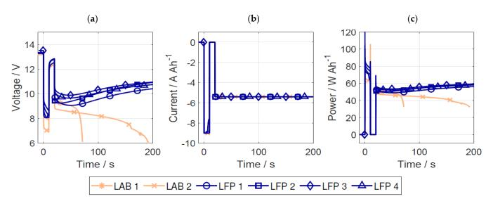
Figure A3. Complete cold-cranking test at -18 °C: (a) voltage, (b) current, and (c) power.
