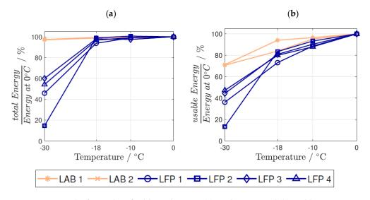
Figure 7. During the first pulse of cold-cranking test (a) total energy and (b) usable energy.
