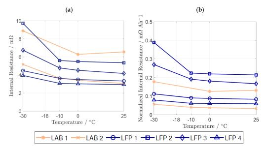
Figure 9. Internal resistance: (a) absolute values and (b) normalized values.
