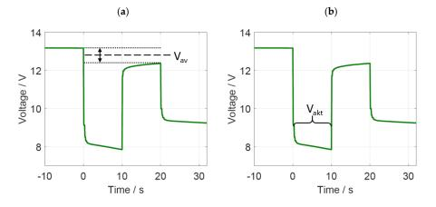
**Figure 6.** Illustration of the voltages used for determining (**a**) the total energy and (**b**) the usable energy during the first pulse of the cold-cranking test.
