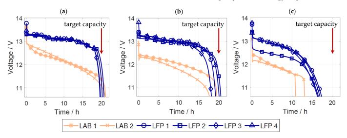
**Figure 1.** C<sub>20</sub> capacity at (**a**) 25 °C, (**b**) 0 °C, and (**c**) -18 °C.
