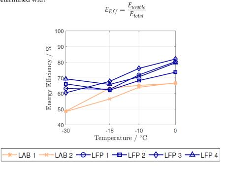
Figure 8. Energy efficiency during first pulse of cold-cranking test.
