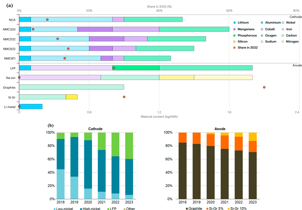
Figure 4. (a) Material content in alternative anodes and cathodes in EV batteries in 2022. (b) Sale share in cathode and anode chemistries, 2018–2023. Low-nickel chemistries are comprised of NMC333 and NMC532, whereas high-nickel ones are NMC622, NMC721, NMC811, lithium nickel manganese cobalt aluminum oxide (NMCA), and lithium nickel cobalt aluminum oxide (NCA). Si-Gr means silicon-doped graphite with a percentage share of silicon. Sales share is measured based on capacity. With permission from [33] for (a) and [34] for (b).
