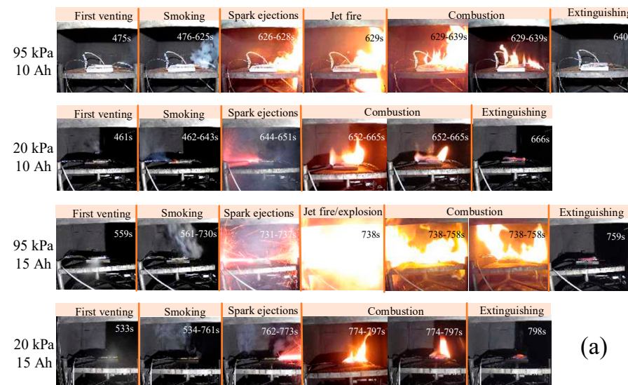
Figure 5. Typical phenomena of LIBs after thermal runaway: (a) group A—single cell in 95 kPa, (b) group A—single cell in 20 kPa, (c) group B—multiple cells in 95 kPa, (d) group B—multiple cells in 20 kPa, (e) 10 Ah pouch cell under 95 kPa, (f) 15 Ah pouch cell under 95 kPa, (g) 10 Ah pouch cell under 20 kPa, and (h) 15 Ah pouch cell under 20 kPa.
