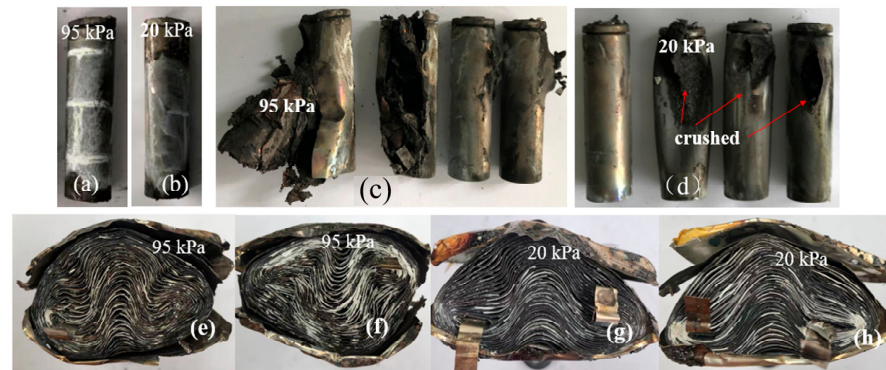
Figure 5. Typical phenomena of LIBs after thermal runaway: (a) group A—single cell in 95 kPa, (b) group A—single cell in 20 kPa, (c) group B—multiple cells in 95 kPa, (d) group B—multiple cells in 20 kPa, (e) 10 Ah pouch cell under 95 kPa, (f) 15 Ah pouch cell under 95 kPa, (g) 10 Ah pouch cell under 20 kPa, and (h) 15 Ah pouch cell under 20 kPa.
