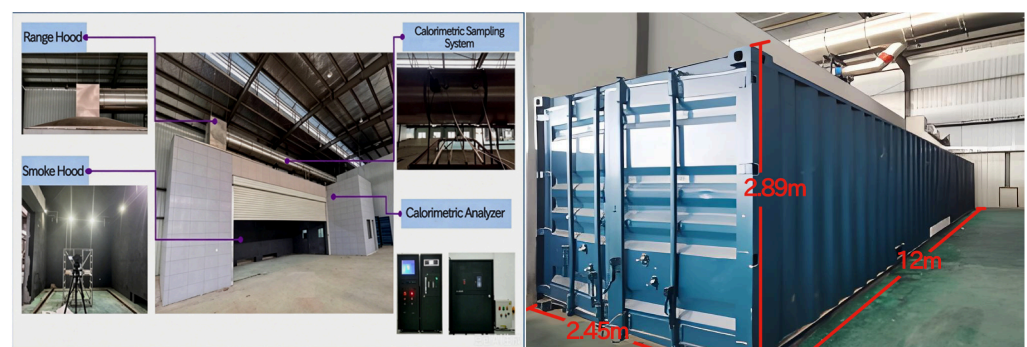
Figure 2. Full-scale fire test platform for lithium-ion battery energy storage system.
