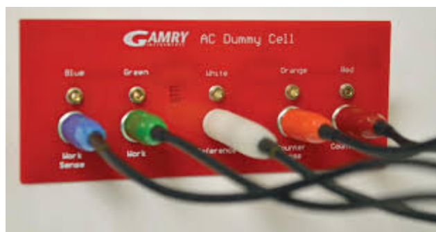
Figure 13. Gamry Interface 5000P connections schematic to the AC Dummy Cell.
