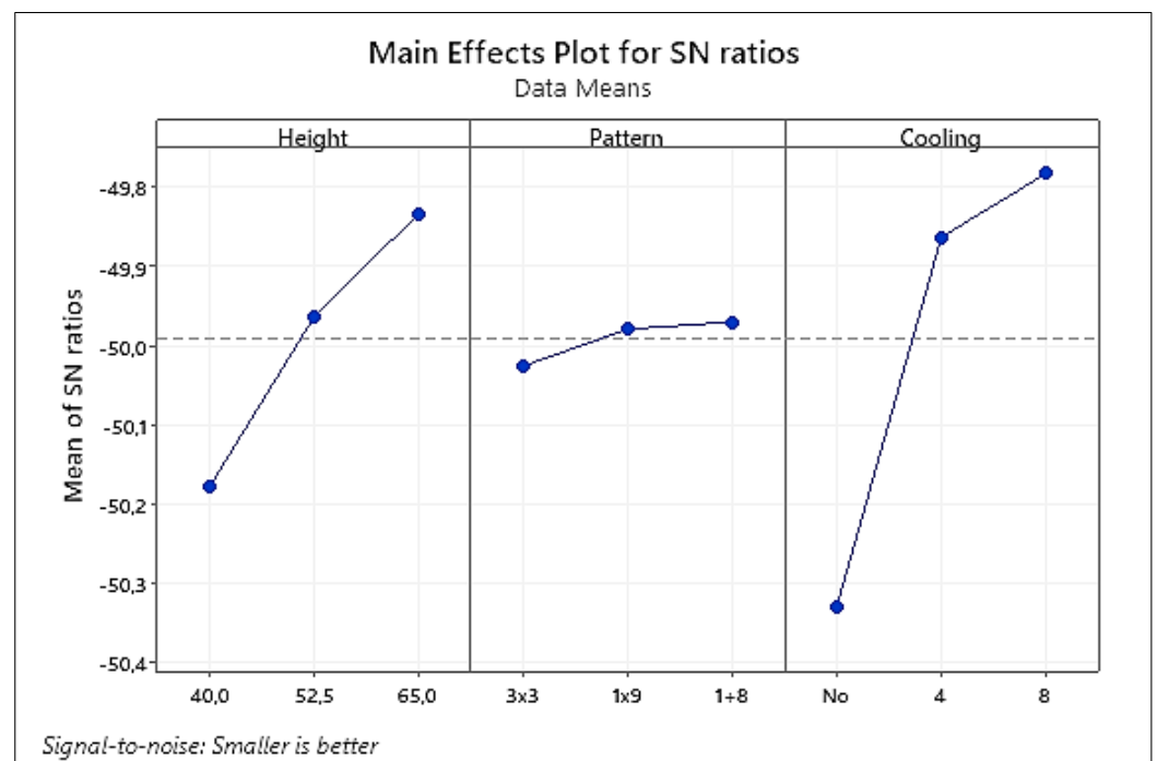
Figure 6. S/N ratio results of the experimental design based on the L9 ( 3^3 ) orthogonal array.
