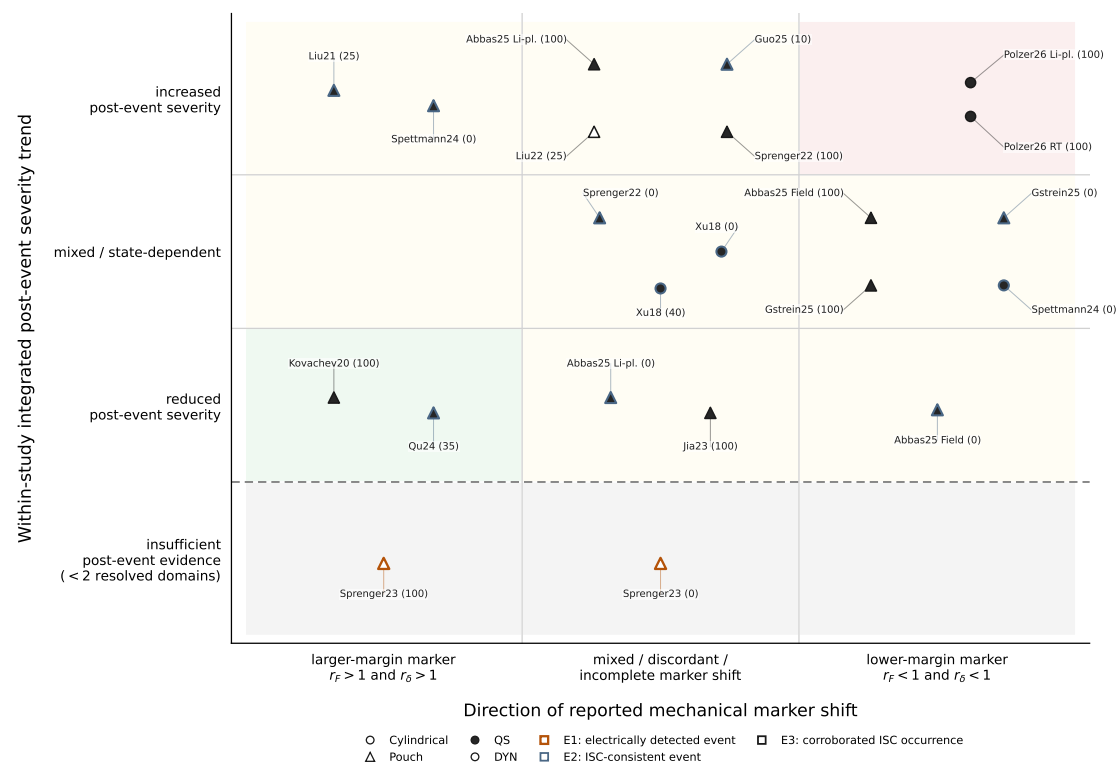
Figure 10. Evidence map linking marker-shift class to integrated post-event severity. Circles and triangles denote cylindrical and pouch cells, respectively; filled and hollow markers denote quasi-static and dynamic loading; and orange, blue, and black marker edges denote evidence tiers E1, E2, and E3. Red and green background fields highlight the unfavorable lower-margin/more-severe and favorable larger-margin/less-severe combinations, respectively; pale-yellow fields denote the remaining classifiable combinations, and the gray field denotes insufficient evidence. Parenthetical values indicate test SoC.
