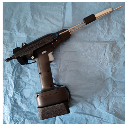
Figure 1. The smart drill system used in the experiments, equipped with an inertial measurement unit and a linear potentiometer.
