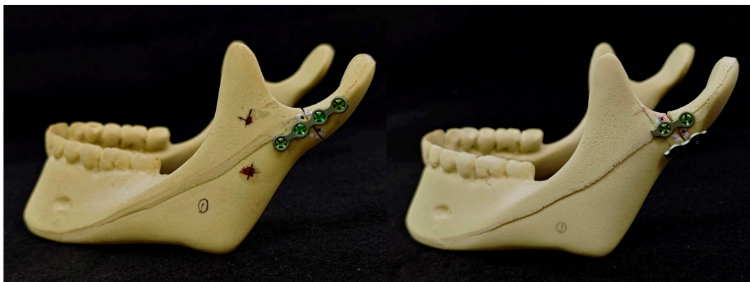
Figure 3. Demonstration of single-long-plate and double-short-plate fixation on Sawbones models.
