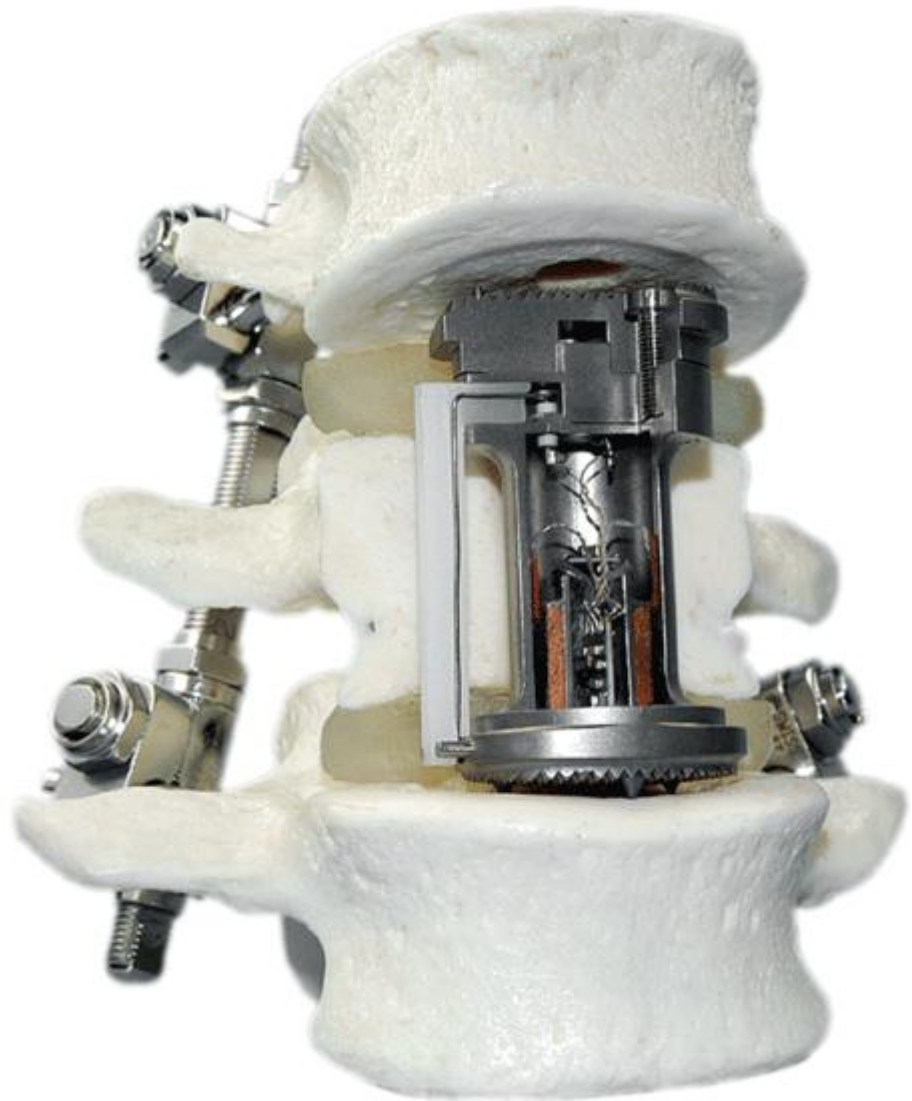
Figure 1. Instrumented vertebral body replacement (SYNEX) modified for in vivo measurement of spinal loads. The implant integrates six load sensors and a 9-channel telemetry transmitter housed within the implant body, enabling continuous recording of three force components and three moment components acting on the vertebral body replacement during daily activities and rehabilitation exercises. Image reproduced from OrthoLoad (Bergmann G, Damm P, eds.; Julius Wolff Institute, Berlin Institute of Health at Charité—Universitätsmedizin Berlin; 2008; http://www.OrthoLoad.com ; accessed December 15, 2025), in accordance with OrthoLoad non-commercial usage policies.
