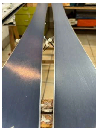
Figure 2. Optical comparison between a prepared ski base ( left ) and an unpolished ski base ( right ). The prepared ski shows a uniform grinding microstructure with a smoother and more reflective surface, whereas the unpolished ski exhibits a rougher texture with irregularities and reduced surface uniformity.
