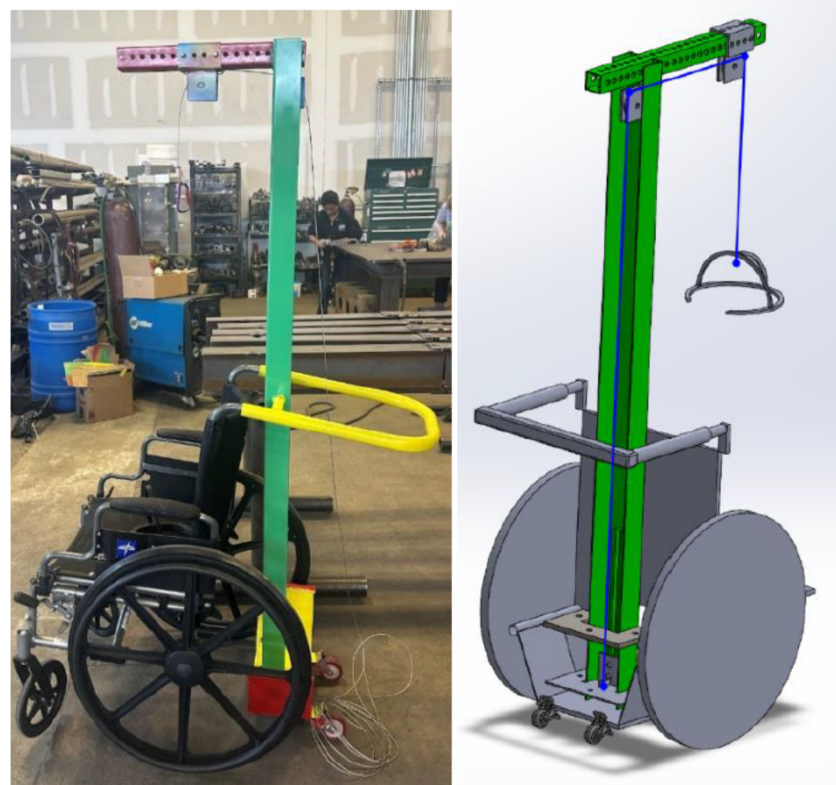
Figure 1. Fabricated prototype and corresponding CAD representation of the proposed halo-gravity traction wheelchair support system.
