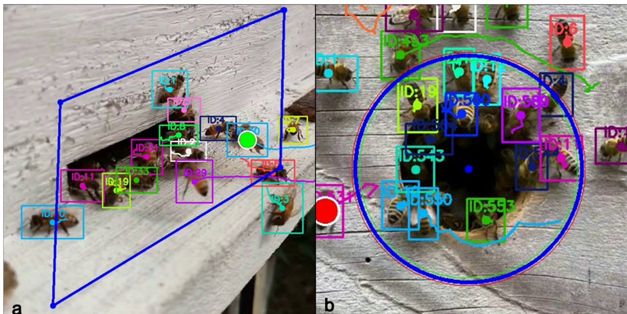
Figure 3. Example configurations of the region of interest (ROI) used for hive entrance monitoring and trajectory-based counting. (a) Polygonal ROI applied to a horizontal hive entrance, illustrating tracked bee identities and direction-aware boundary crossings. (b) Circular ROI configuration used for a vertical hive entrance, demonstrating stable multi-object tracking and aggregation of entrance and exit events.
