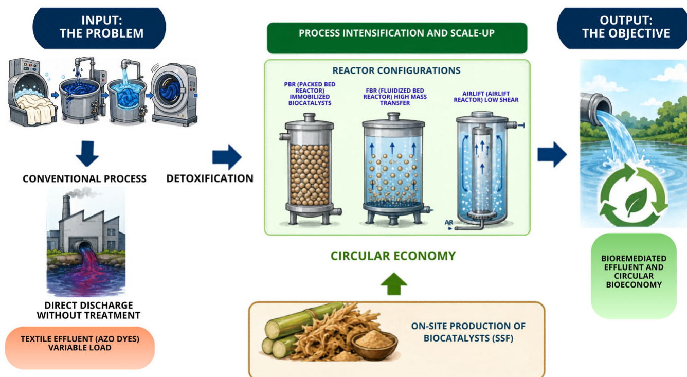
Figure 3. Reactor configurations for textile wastewater bioremediation using solid-state fermentation-derived biocatalysts. Engineering perspectives on textile wastewater bioremediation: overview of input challenges, process intensification parameters, and scaling-up via diverse reactor configurations. The blue arrows indicate the sequential process flow, from the generation of textile wastewater and detoxification to treatment in different reactor configurations and the production of a bioremediated effluent. The green arrows and circular symbol represent the integration of on-site solid-state fermentation (SSF)-derived biocatalyst production with the circular economy concept, highlighting biomass valorization, resource recirculation, and closed-loop industrial implementation. The integration of on-site SSF provides a cost-effective pathway for biomass valorization, resulting in detoxified effluents and supporting the transition toward a circular bioeconomy.
