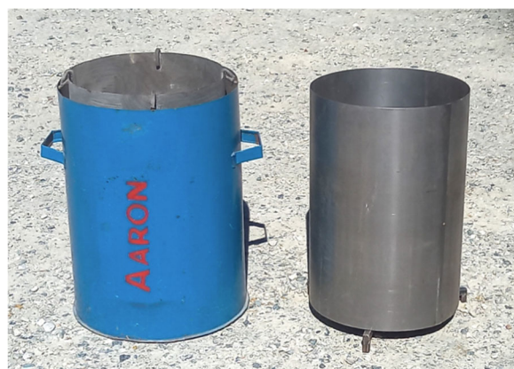
Figure 7. A lateral view of the original Aaron stove (left) and the Aaron light stove (right).
