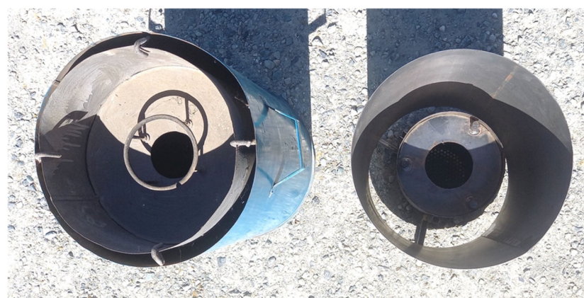
Figure 8. The view from above of the original Aaron stove (left) and the Aaron light stove (right). To better sustain the pot, an iron ring can be welded to the three supports, like in the center of the original stove on the left.
