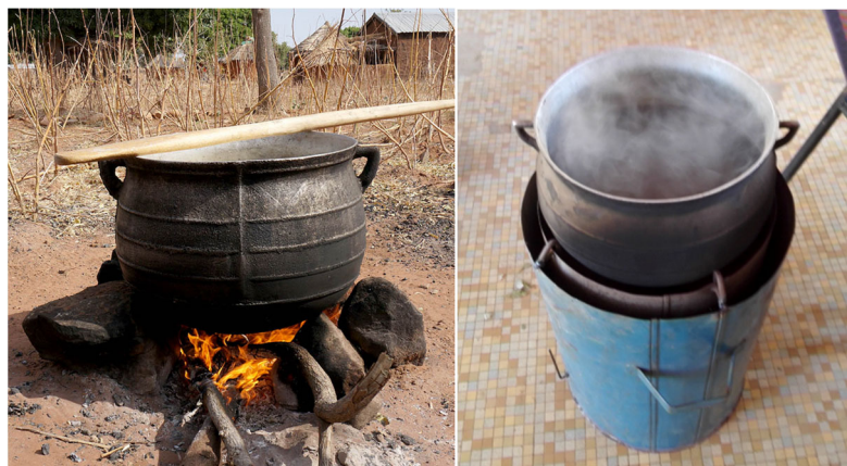
Figure 4. A traditional aluminum round pot, number 5, on a stone fire (left) and during testing on the Aaron stove (right).
