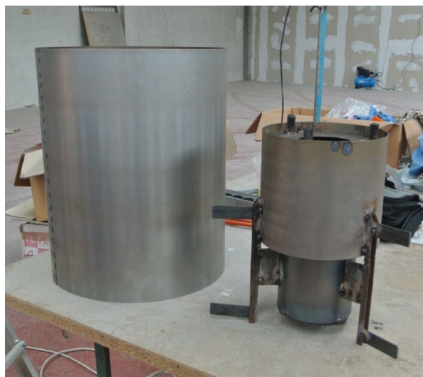
Figure 11. The Aaron light stove with the external cylinder removed. On the left is the external cylinder, on the right is the second (medium) cylinder, and inside it is the inner cylinder and the reactor, with its lower part visible.
