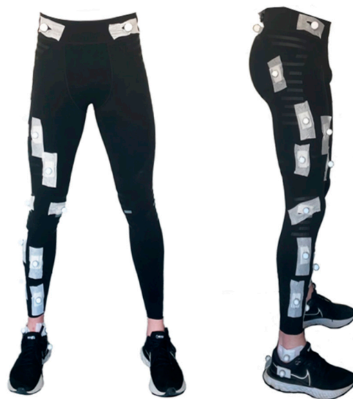
Figure 2. Supportive tension brace with marker set.
