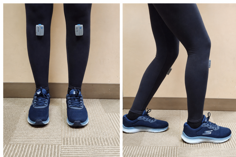
Figure 1. Location of the shank-mounted IMU. The (left) panel shows the frontal view and the (right) panel shows the sagittal view. The sensor was placed on the anterior and slightly medial aspect of the tibia.
