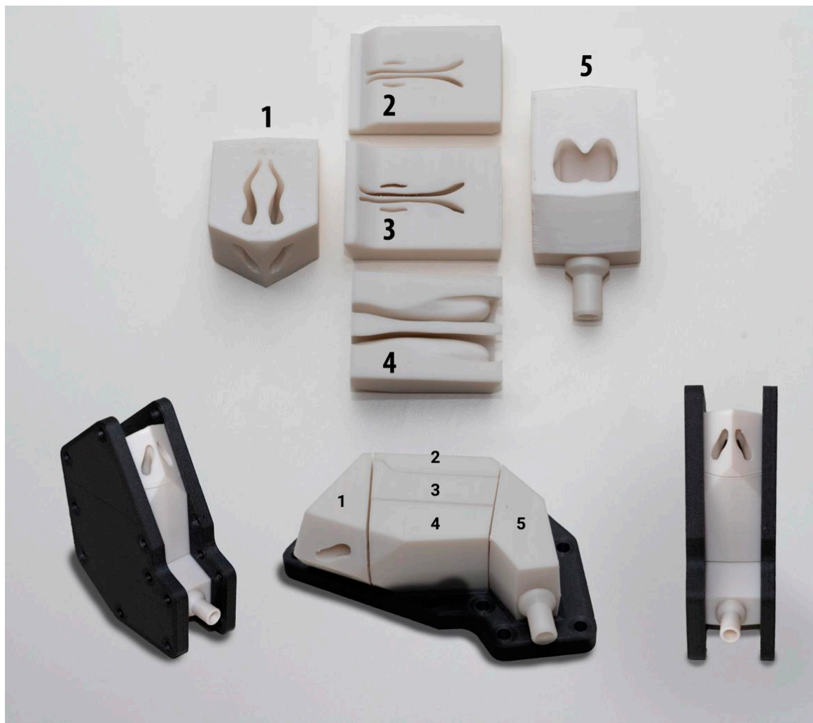
Figure 5. Assembled 3D-printed nasal cavity model in the fixation device and individual parts of the model. Nasal vestibule (Region 1), Olfactory region (Region 2), Middle and upper turbinates (Region 3), Lower turbinate (Region 4), Nasopharynx (Region 5).
