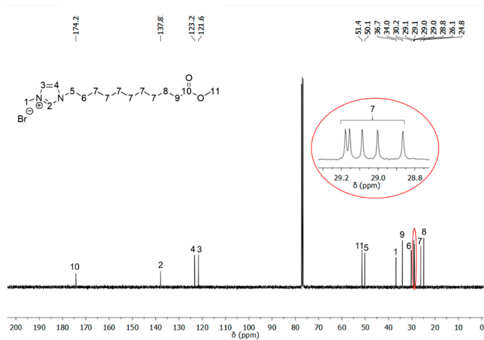
Figure S4. ^{13}\text{C} NMR spectrum of 3-(11-methoxy-11-oxoundecyl)-1-methyl-1H-imidazolium bromide (2).
