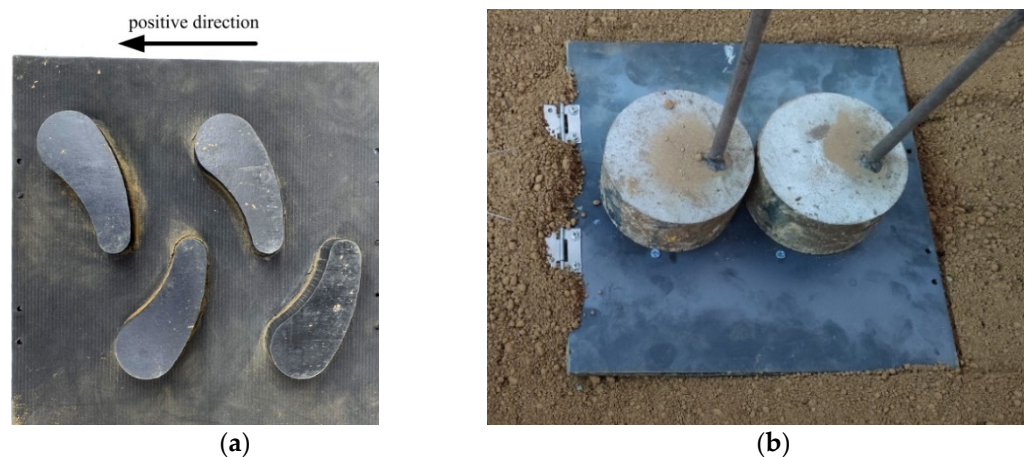
Figure 9. Test direction and load: (a) pattern direction; (b) apply 100 N load.
