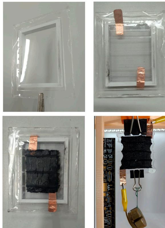
Figure 6. The step-by-step fabrication process of the DEA.
