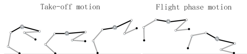
Figure 6. The process of quadruped robot with a flexible spine.
