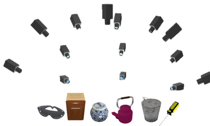
Figure 3. Color and depth images with poses are randomly captured on the hemisphere by controlling the camera in the simulation environment.
