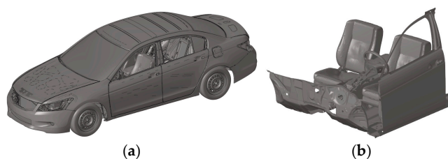
Figure 4. Vehicle FE Model: (a) Accord full-scale model, (b) simplified sled model.
