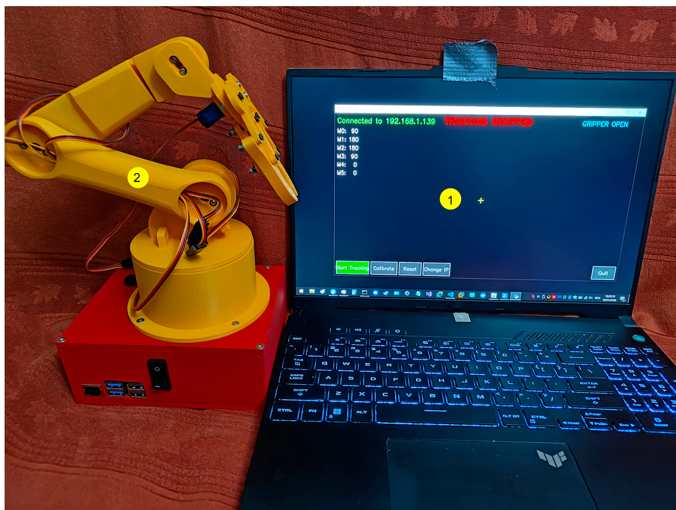
Figure 1. System overview of the interactive teleoperation setup: 1. operator-side GUI for vision-based hand tracking and command generation. 2. articulated robotic arm platform executing the received commands.
