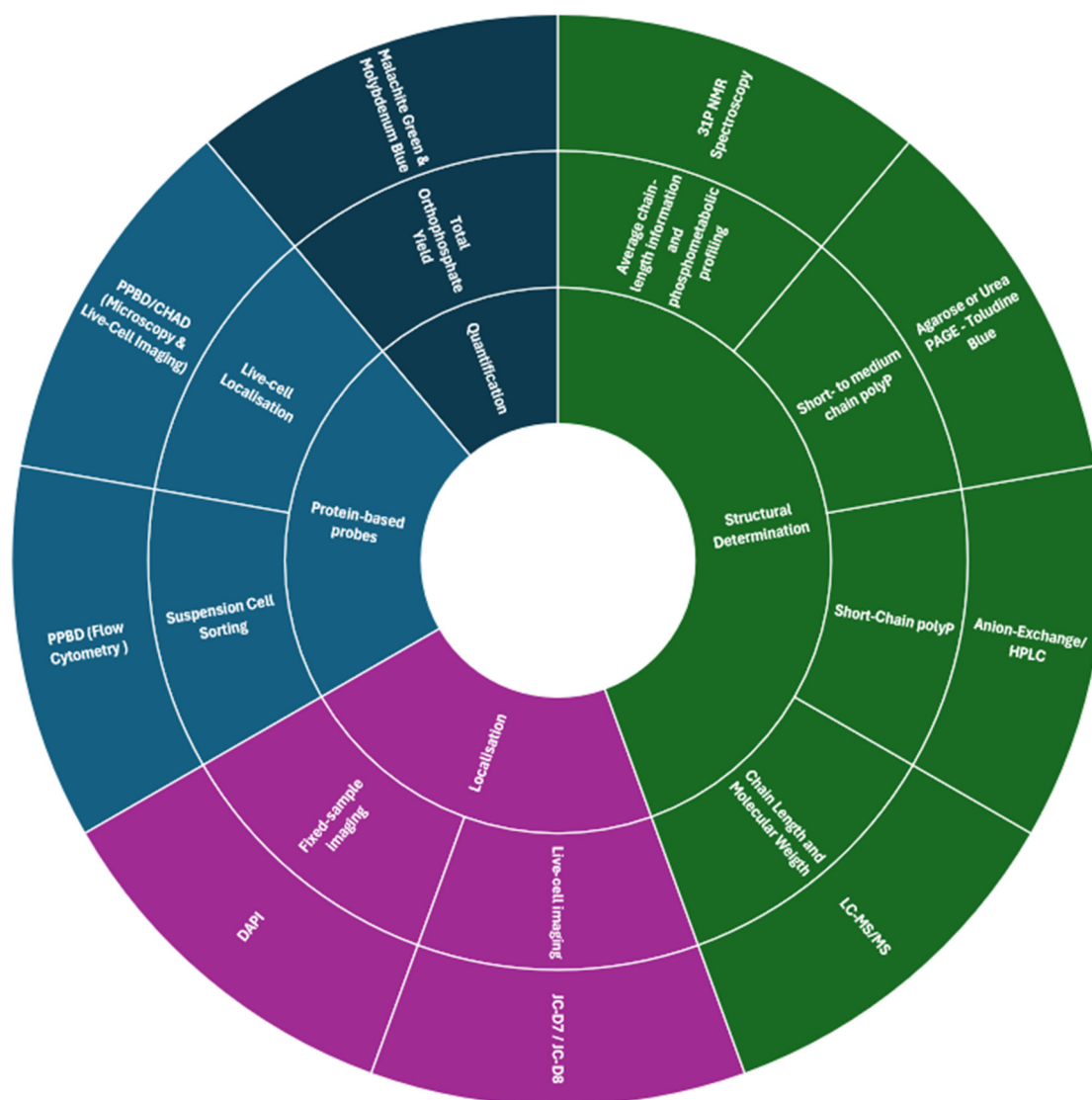
Figure 1. Comprehensive framework for polyP characterisation and detection methodology. The classification system is organised into a concentric, multi-layered sunburst hierarchy based on how each method interacts with polyP. The Inner Ring divides the analytical toolkit in Protein-Based Probes, Localisation, Structural Determination, and Quantification. The Middle Ring maps these approaches to their precise physiological and structural applications, including average chain information and phosphometabolic profiling, short-to-medium-chain polyP, chain length and molecular weight, live-cell imaging, and total orthophosphate yield. The Outer Ring shows the specific, actionable techniques available to detect polyP (e.g., Malachite Green, Molybdenum Blue, Phosphorus-31 Nuclear Magnetic Resonance ( ^{31}\text{P} NMR) spectroscopy, agarose or urea–polyacrylamide gel electrophoresis (PAGE)–Toluidine Blue, Anion-Exchange, high-performance liquid chromatography (HPLC), LC/MS-MS (liquid chromatography–tandem mass spectrometry), JC-D7/JC-D8, polyphosphate-binding domains (PPX_Δ12/PPBD), conserved histidine \alpha -helical domain (CHAD).
