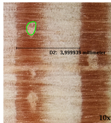
Figure 2. Anatomical characteristics of P. pinaster observed in the transverse plane. The boundary of the resin duct is highlighted in green, while the black line indicates the measurement of growth ring width. Magnification = 10 \times .
