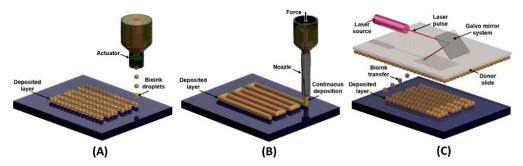
Figure 2. Schematic models for (A) inkjet, (B) extrusion, and (C) laser-assisted bioprinting techniques.
