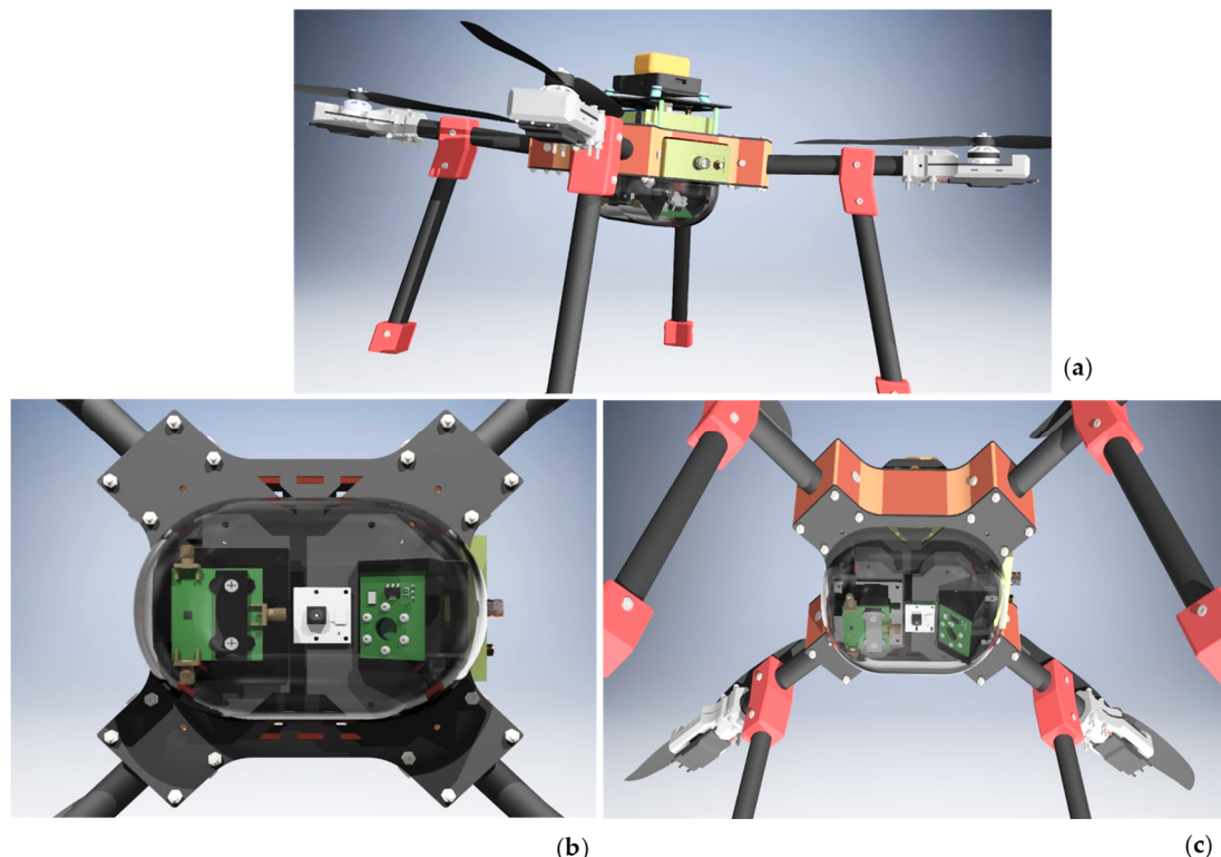
Figure 10. Conceptual design of a drone-based York DF Photon Counting Biosensor. (a) Top image shows the full view of the drone-integrated York DF Photon Counting Biosensor with PCS121 electronics, SiPM bias supply and amplifier integrated into the drone body; (b) Left image reveals the belly view of the optical elements of the device within dome, including the SiPM, target camera in the center, and excitation LED; (c) Right image displays a hovering drone bottom view. Credit: Biosensor integrated drone design by Haktan Yağmur [54].
