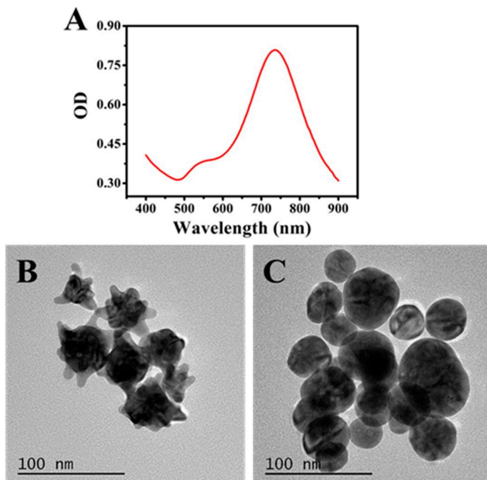
**Figure 1.** (A) UV-Vis spectrum of AuNS; (B) TEM images of AuNS before etching and (C) after etching.
