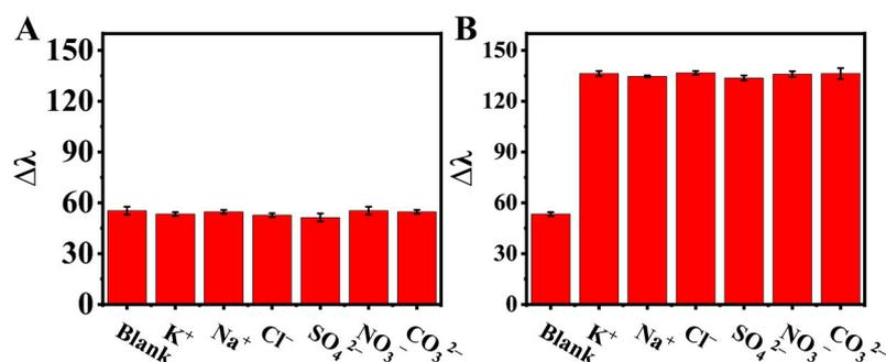
**Figure 5.** (A) The effect of (K<sup>+</sup>, Na<sup>+</sup>, Cl<sup>-</sup>, NO<sub>3</sub><sup>-</sup>, SO<sub>4</sub><sup>2-</sup>, CO<sub>3</sub><sup>2-</sup>) on the selectivity detection of H<sub>2</sub>O<sub>2</sub>. The concentration of H<sub>2</sub>O<sub>2</sub> was 26.67 μmol L<sup>-1</sup>. (B) The interference study for detecting H<sub>2</sub>O<sub>2</sub>.
