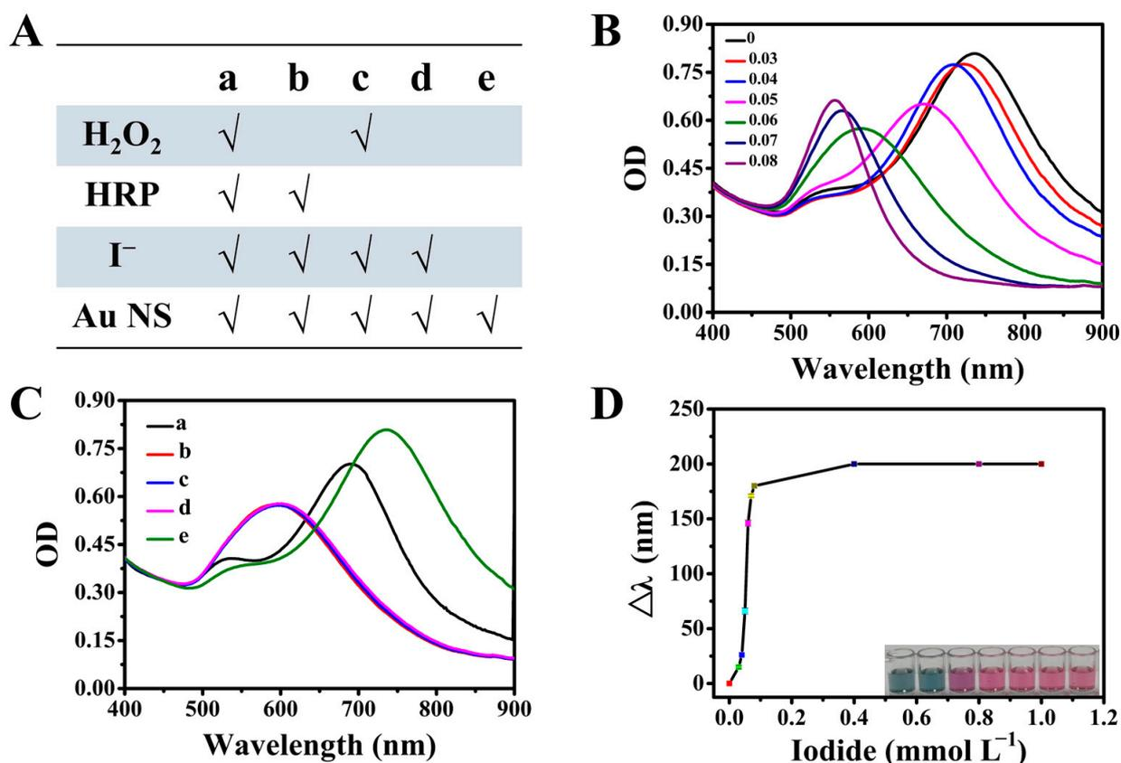
**Figure 2.** (A) Table of the solutions (a, b, c, d, e) with different components for the etching of AuNS. (B) The corresponding UV–Vis spectra of AuNS after etching with different components. (C) UV–Vis spectra of AuNS after etching by different concentrations of  $\text{I}^-$ . (D) The relationship between etching degree and  $\text{I}^-$  concentration. Inset is the color change with varying degrees of etching.
