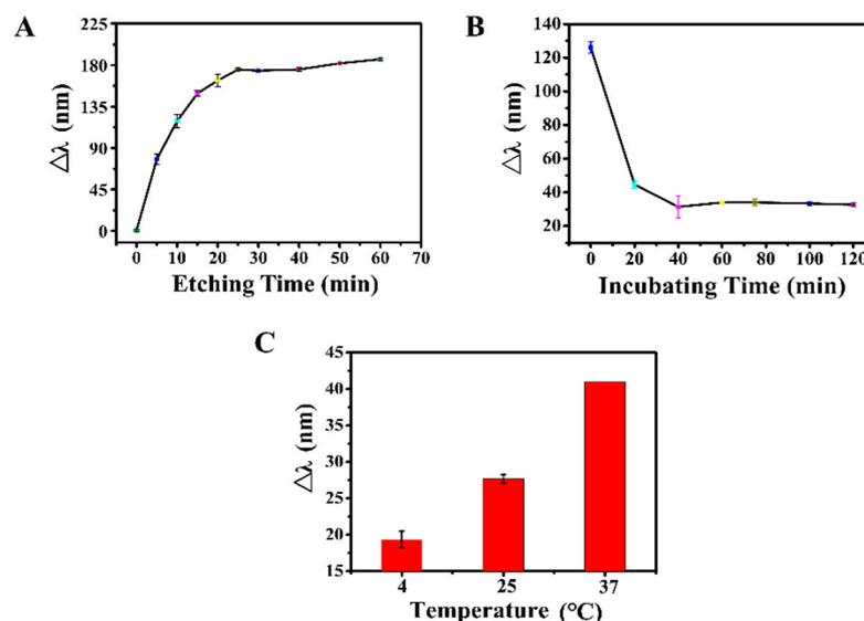
**Figure 3.** Optimization of (A) time for  $\text{I}^-$  etching of AuNS at 37 °C; (B) response time for the reaction between HRP and  $\text{H}_2\text{O}_2$ ; (C) reaction temperature.
