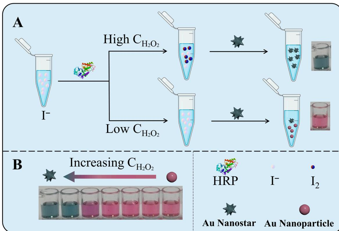
**Scheme 1.** Schematic illustration of iodide-mediated etching of Au NS for  $H_2O_2$  detection (A) and color changes with increasing  $H_2O_2$  (B).
