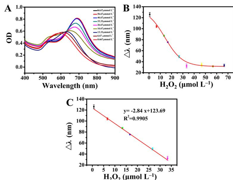
**Figure 4.** (A) UV-Vis spectra of iodide-mediated etching of AuNS in the presence of  $\text{H}_2\text{O}_2$  with different concentrations. (B) The responses of  $\Delta\lambda$  to different concentrations of  $\text{H}_2\text{O}_2$ . (C) Linear relationship between  $\Delta\lambda$  and  $\text{H}_2\text{O}_2$  concentration.
